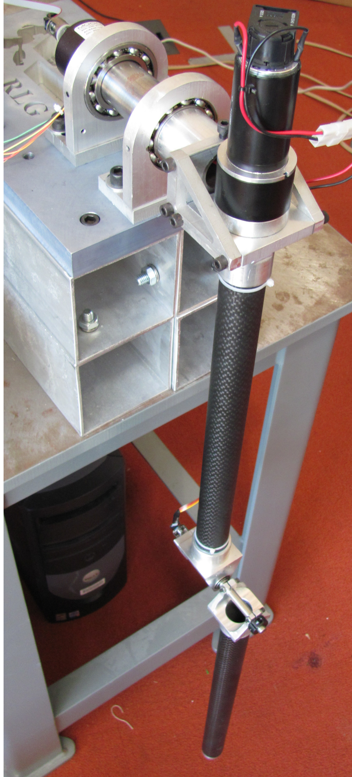
Figure 2-2: The acrobot built previous to the design of the compass gait walker. The motor on the first link is connected to the elbow by a long driveshaft. The encoders in question are located on the back of the motor at the top and on the elbow near the bottom of the picture.
