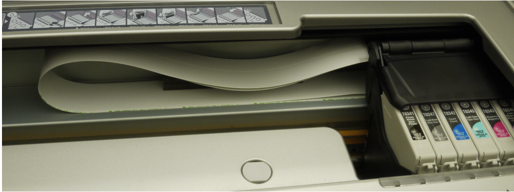
Figure 2-9: The cable which connects to the moving carriage in an inkjet printer was the design inspiration for the similar mechanism in the robot's feet.
