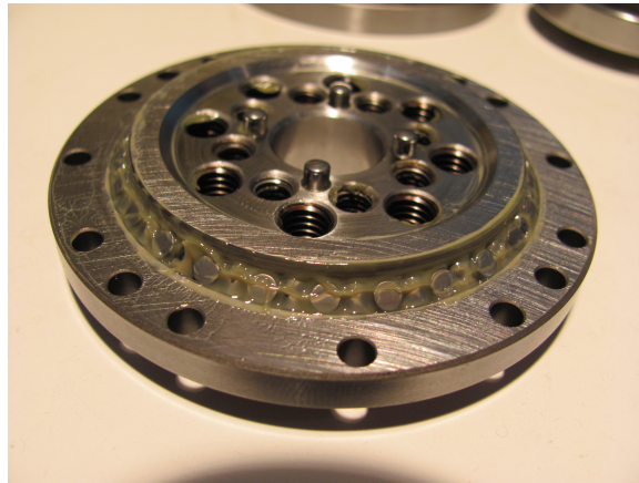
Figure 2-16: The cross roller bearing inside the robot's Harmonic Drive gearbox.
