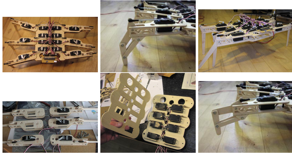
Figure 1.8: Webx hexapod design. This project is found on the Internet. This robot uses Atmel AT90S8515 processor at 8 Mhz and some RC components. This is a hobby project
