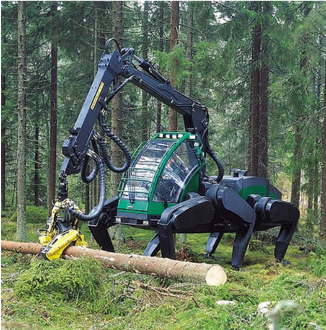
Figure 1.11: Timberjack, a walking machine project by Pulstech. The control and walking procedure is done by an intelligent computer.
