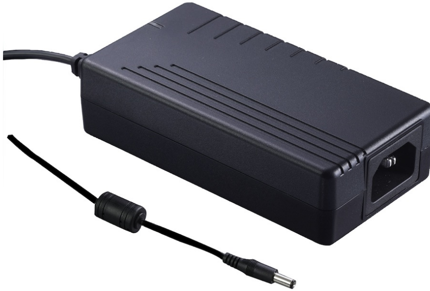
Figure 2.6: Shanjing Power Supply, input:100-240 Volts and 1.2 A 50/60Hz, output:5V 7A
